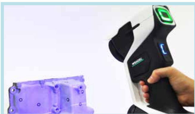
Single line scanning mode for deep holes
