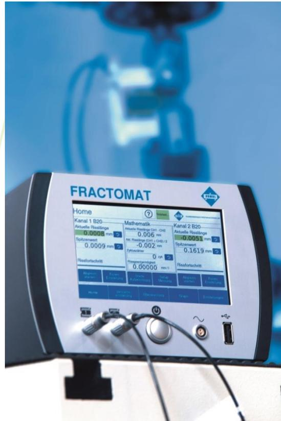
Measuring the crack length is in a large number of tests in fatigue or in fracture mechanics an essential procedure. The test configuration requires a high accuracy to receive exact results.
