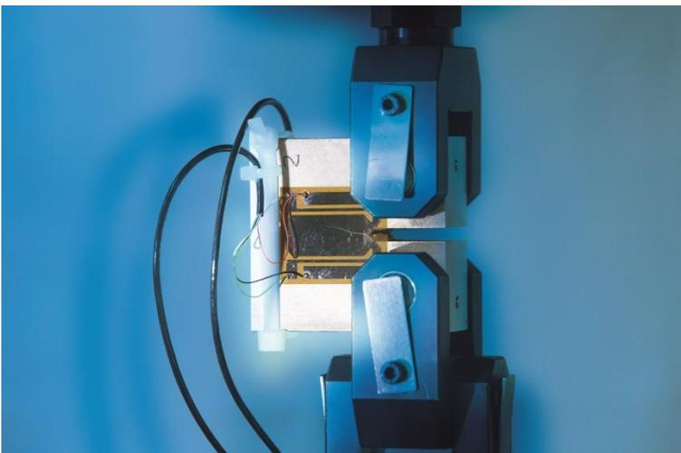
*Krak Gages bonded to a CT sample during fatigue crack propagation test*
