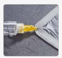
The new Elcometer 135C Bresle Test Patches have a thicker foam surround compared to traditional patches, allowing easier insertion of the syringe.
