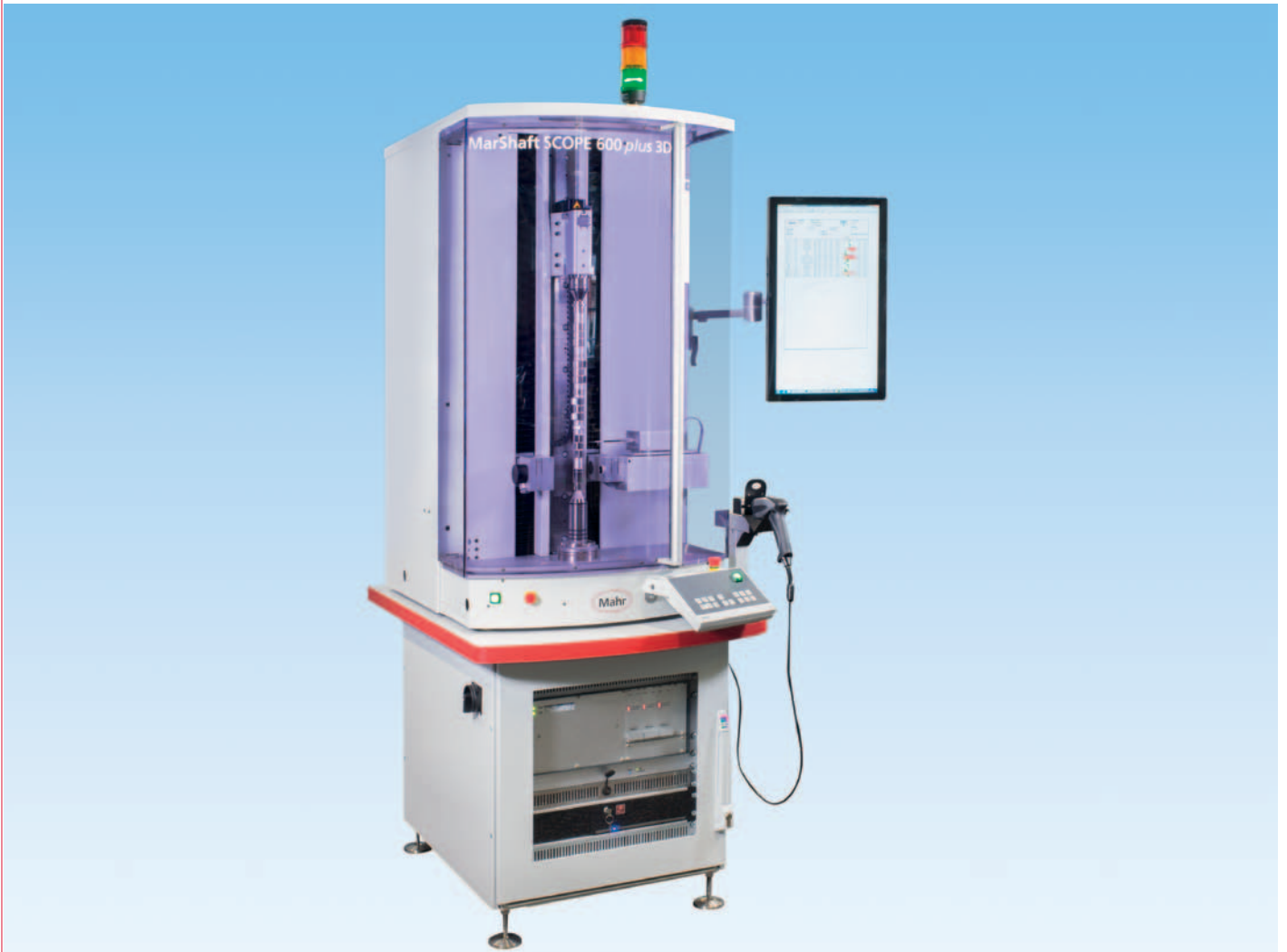
MarShaft SCOPE 600 plus 3D Optical and Tactile Shaft Measuring Machine for Camshafts
